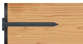
Fig. 1. Fastening of the roof paper to the timber
