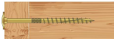
Fig.1. Perpendicular screw-in connection
