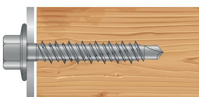
**Fig. 1.** Fastening of steel sheets to timber supporting structures.
