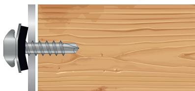
**Fig. 1.** Fastening of roof works and profiled roof metal sheets to wooden structures.
